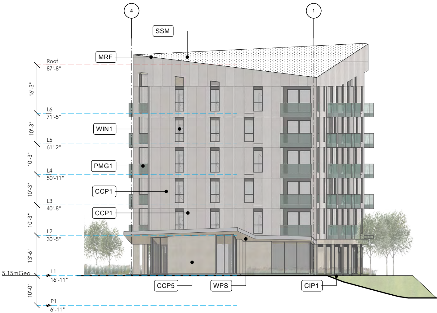
North Elevation - Interior Amenity
