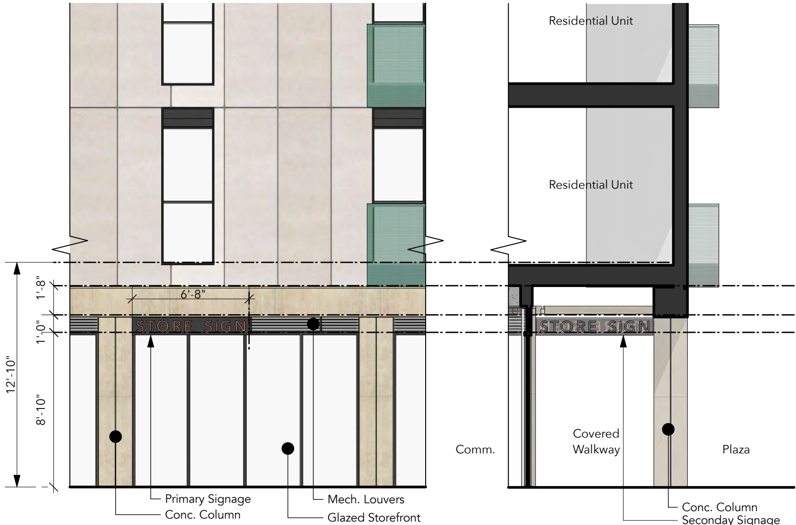
Partial elevation of typical commercial facade
