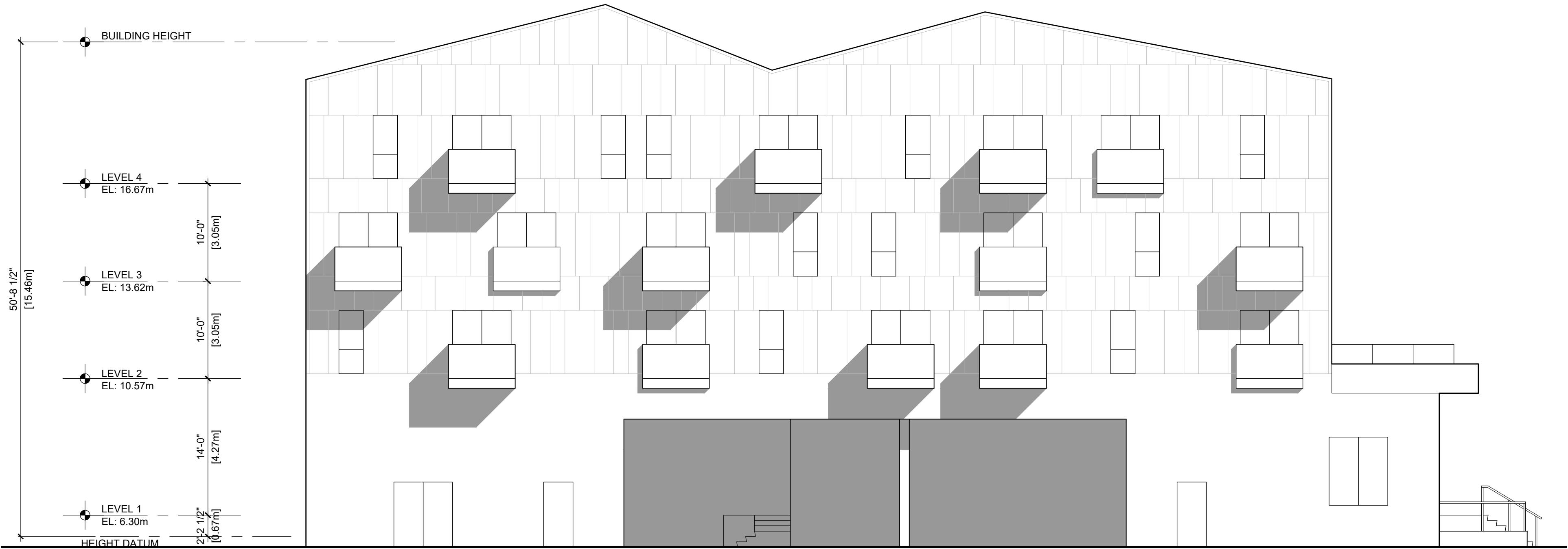
3 BUILDING 2 EAST ELEVATION SCALE: 1/8"=1'-0"
