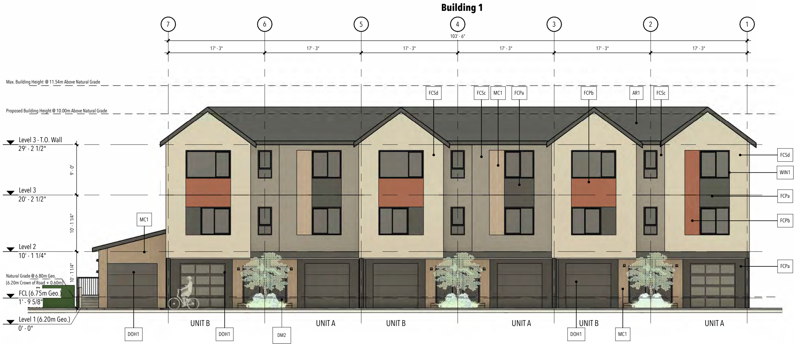
Typ. East Elevation - BLDG's 1 & 6
